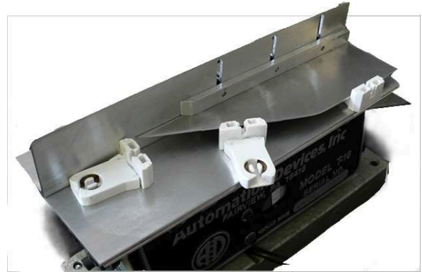
Fig. 1. Reconfigurable modular hardware implementation of the blade device, mounted on a vibratory device. Three parts are on the track, moving from left to right, of which the rightmost is output. The “knocker” wiper (section IV) is the triangular shape attached to the side of the rightmost end of the track.
